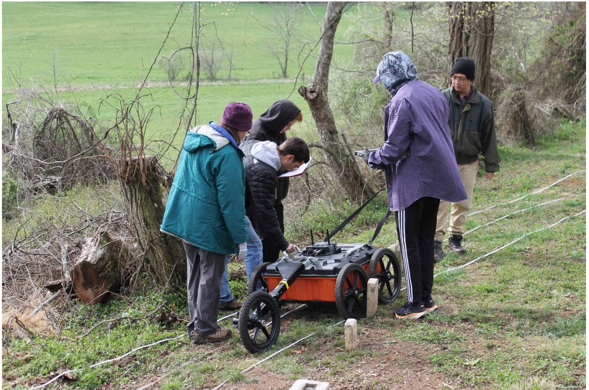
Above: The GPR Team with the GPR Deployed, imaging everything beneath the surface to a preset depth (It has a maximum depth range of 70 feet, but we didn't need that setting thank goodness!)
