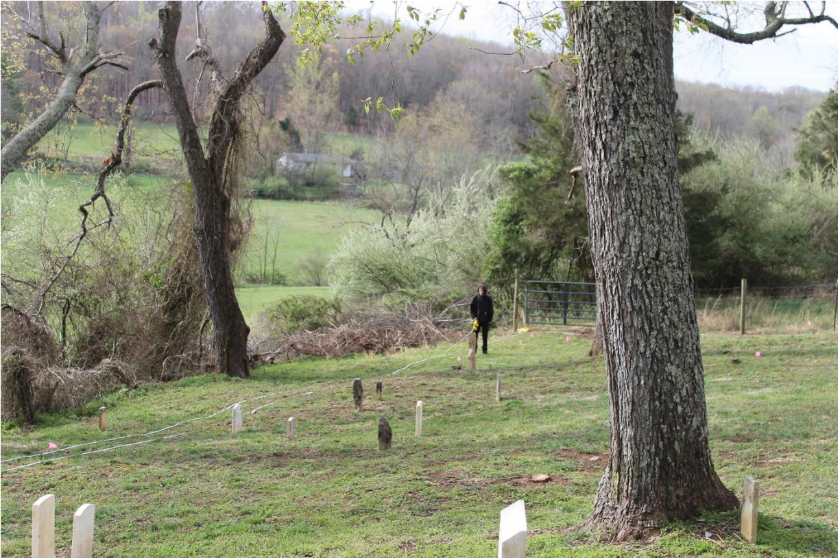
Above: Establishing and Setting the GPR Travel Lines
